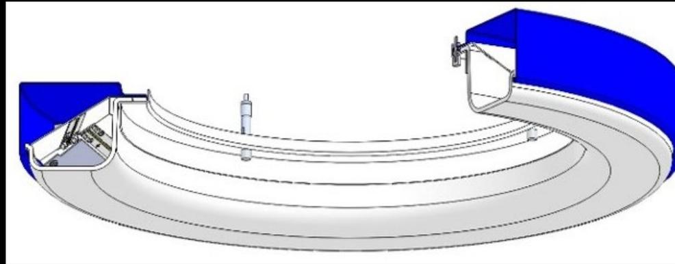
precision CNC spun .063" aluminum housing w/ rolled bottom edge for added strength
